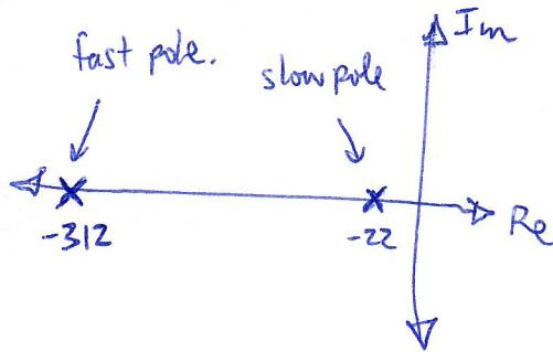
It turns out the fast pole is due mostly to the electrical part of the motor ( $R$  and  $L$ ).
