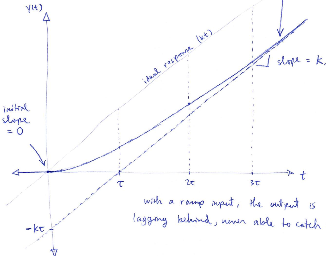
with a ramp input, the output is lagging behind, never able to catch up.
